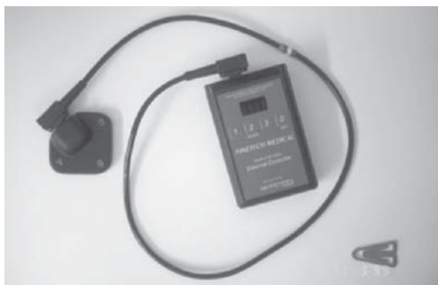
Fig. 14.3 A sacral anterior root stimulator used to 'drive' micturition following a deafferentation (external components).
